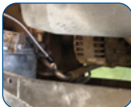
Leak from low pressure connection.
