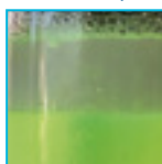
Refrigerant and additive contaminated by water
